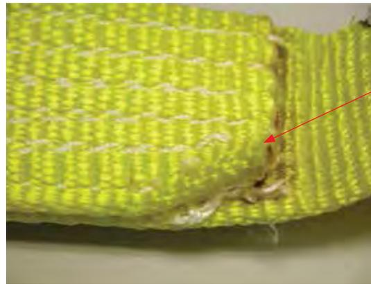
**THE DAMAGE: Knots** compromise the strength of all slings by not allowing all fibers to contribute to the lift as designed. Knots may reduce sling strength by up to 50%.
